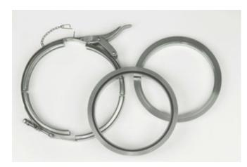
FLW clamp connections as a clamping band with quick release and lock. Incl. clamping device on the joint as well as mounted profile segments Separately: Tongue and groove flange with inserted O-ring.
