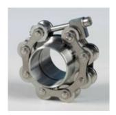
The FL-Ultra clamping roller chain made of stainless high grade steel on equally stainless conical flanges is a reliable solution. The tube ends are placed against each other by hand after inserting a forced centring sealing ring. The clamping roller
